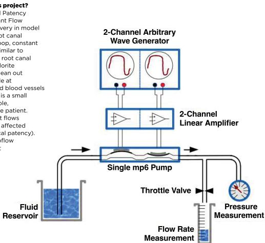
This diagram illustrates the benchtop setup for pump controller development in single-pump configuration.
