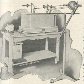
ing, is one of the most powerful machines manufactured, doing X-Ray work with exposure of seconds instead of minutes, as with the old static machines. Negatives can be made of hand, foot or leg in one second, and of the chest, abdomen and hip in from ten to thirty seconds. This makes a .most valuable addition to the diagnostic equipment owned by the A. S. O. A new dark room, in has been constructed and equipped for the rapid development of the X-Ray prints.
