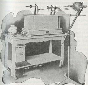
ing, is one of the most powerful machines manufactured, doing X-Ray work with exposure of seconds instead of minutes, as with the old static machines. Negatives can be made of hand, foot or leg in one second, and of the chest, abdomen and hip in from ten to thirty seconds. This makes a most valuable addition to the diagnostic equipment owned by the A. S. O. A new dark room, in has been constructed and equipped for the rapid development of the X-Ray prints.
